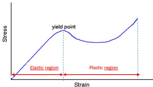
The slope of the plotted curve, gives us immediately a good idea of the plasticity of the material. When the slope of the plot is steep (= high Tensile Modulus), the material resist very well deformation. But when the slope is gentle, the plastic has a low Tensile Modulus, which means it will be easily deformed.
