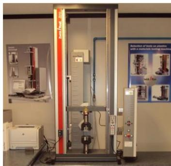
First of all, the determination of the ultimate tensile strength and the strength at break, are the most common definitions used to specify plastics. Hereby we cannot only analyze thin plastic sheeting, but also all kind of plastic package materials. These measurements are performed according different ISO and ASTM standards, depending on the type of product and depending on the information you want to achieve.
