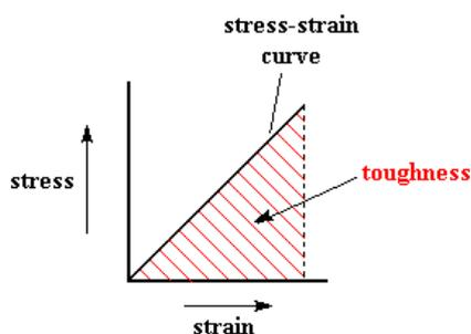
This differs from the force that is needed to break a sample! A strong sample is not necessary tough and vice versa.
