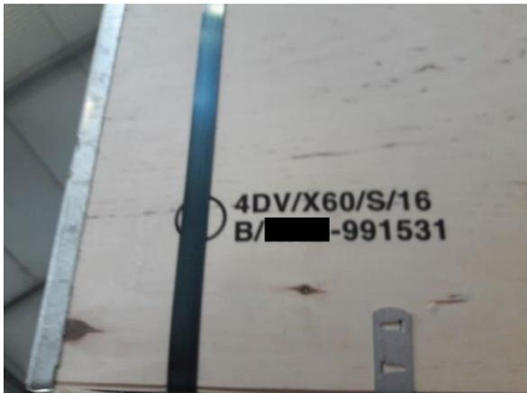
*Here the UN mark is completely correct, but unfortunately the UN symbol is covered by the strap, what makes it invalid.*
